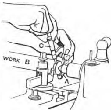
FIG. 8. — MEASURING WORK IN THE LATHE WITH MICROMETER.
